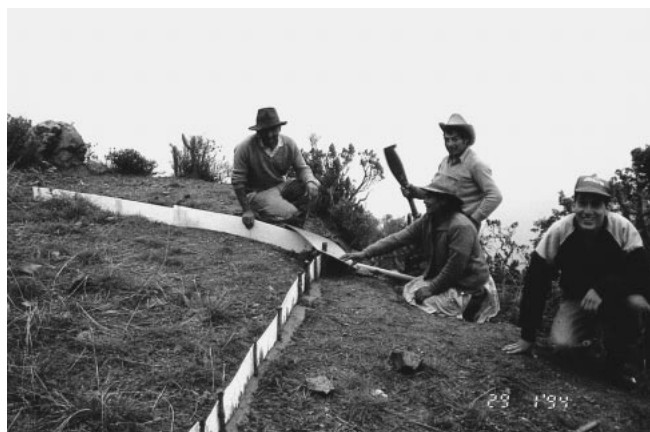
FIGURE 4 Experimental plot for measuring run-off and sediment yield on an abandoned terrace. (Photo by authors)
